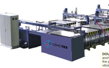
**DOUBLE ANCHORAGE:** pallets anchorage by two positions while the printing process avoiding any vibration and assuring precision of +- 0,02mm
