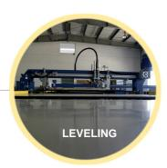
PALLET AUTOMATIC LEVELLING SYSTEM, in height and horizontal. It permits to print several levels very accurate.
